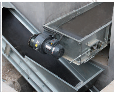
Transverse Manure Conveying System
