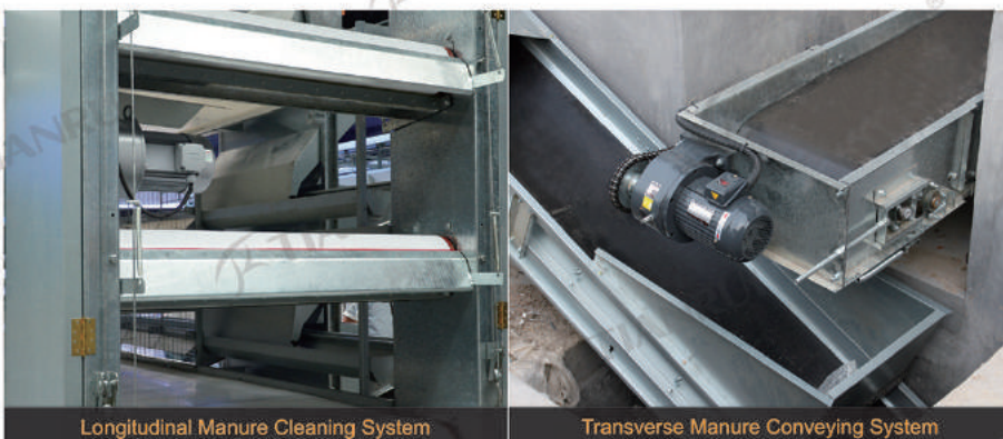
Longitudinal Manure Cleaning System
