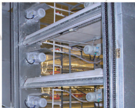
Longitudinal Manure Cleaning System
