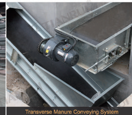
Transverse Manure Conveying System
